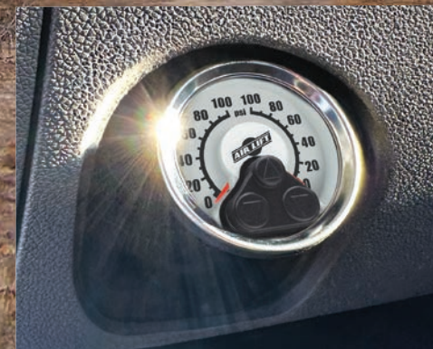
Compact models can be mounted in-dash or with the included mounting pod (dual-path gauge pictured left), while the panel model comes pre-mounted for quick under-dash installation.
