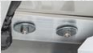
Bolt Plate Reinforcement for Aftermarket Rack System (Option)
